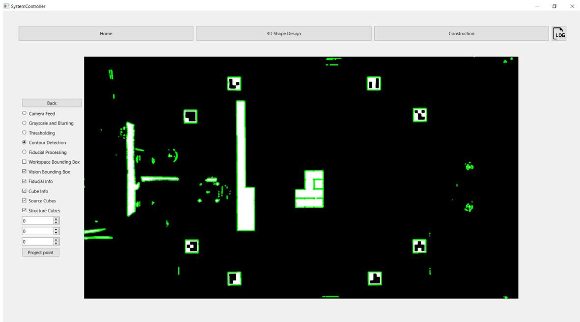
Figure 26. System control software vision view screen with contour step displayed.
