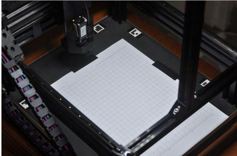
**Figure 17. Placement of grid in the robot's workspace to facilitate the measurement of the z-axis rotational repeatability.**
